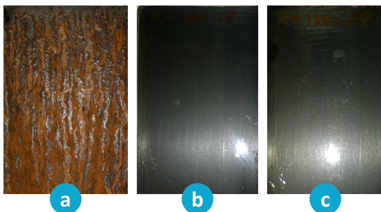
Figure 1. (a) Uncoated carbon steel plate after 168 hours of salt fog exposure (b) Carbon Steel Plate coated with RS50 (4 coats) before exposure and (c) Carbon Steel Plate coated with RS50 (4 coats) after 500 hours of salt fog exposure.
